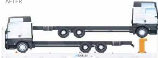
truck chassis x 2units on 40'flat rack container
