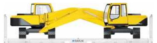
excavator (22ton) x 2units on 40'flat rack container
