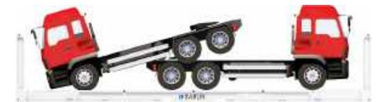
tractor head (6x4) x 2units on 40'flat rack container
